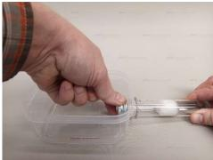
Tip some sand-clay mixture (½ teaspoon approx.) into the tube. Ensure that the marked side stays up.
